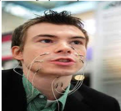
Figure 2-Electrographic sensors attached to the face.
